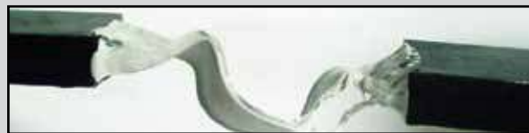
■ Traditional sealant has stringy, putty like substance and easily pulls apart and breaks.
