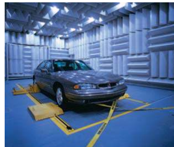
Facilities at the 30 000 m 2 test centre in the USA include sound-reflecting and anechoic chambers, where tests are carried out under simulated real-life conditions during the development phase
